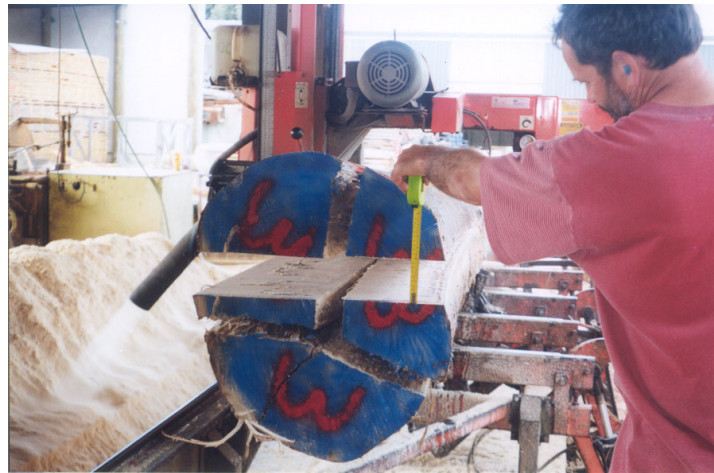
Figure 2: E. nitens 15 yr old - flitch movement during sawing
