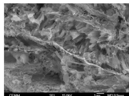
fig 1. SEM image of particles PG bonding from the plasticized sulfur in SPC 26-40 sample.
