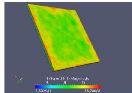
Fig 3. Radon exhalation rate obtained for different surface points of plate (1 x 1 x 0.04 m<sup>3</sup>) of SPC 30-50 samples.
