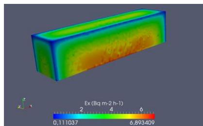
Fig 2. Radon exhalation rate obtained by modelling a specimen of 0.004 x 0.004 x 0.16 m<sup>3</sup> made with SPC 30-50 sample.
