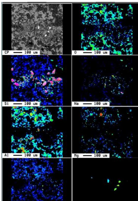
fig 4. BSE image (CP) and WDS X-ray maps showing the distribution of different elements. Color scale indicates the relative number of X-ray counts per pixel (low: blue, med: green-yellow, high: red-pink).
