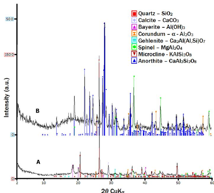
fig 2. X-ray diffraction patterns of green (A) and sintered (B) aggregates.
