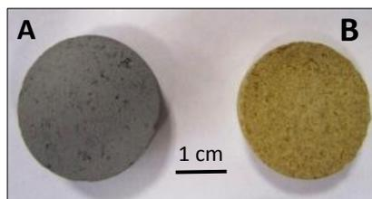
fig 1. Green (A) and sintered (B) aggregates.
