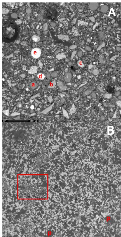
fig 3. BSE images of green (A) and sintered (B) aggregates. a: corundum, b: quartz, c: K-feldspar, d: calcium silicate, e: Si-Fe-Al-O phase; p: pore. Red zone in B is showed in fig 4.
