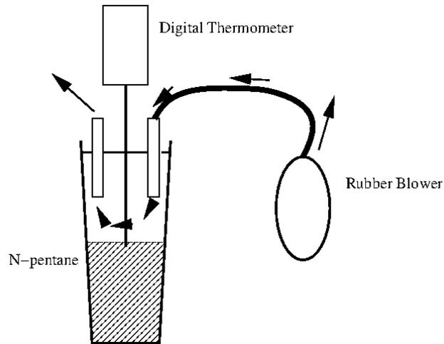
Figure 1: Scheme of the chilled mirror dewpoint hygrometer.
