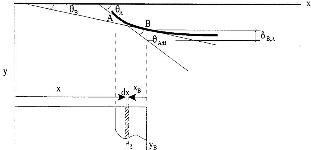
$$\theta_{A-B} = \theta_A - \theta_B = \int_A^B \frac{M_z}{E \cdot I_z} dx = \frac{S^{M_{A,B}}}{EI_z} \quad \delta_{BA} = \int_A^B \frac{M_z \cdot x_B}{E \cdot I_z} dx = \frac{Q_B^{M_{A,B}}}{EI_z}$$
